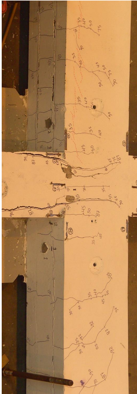
a) Experimental (at failure, the hidden lines are the cracks that happened between the yielding load and failure)
