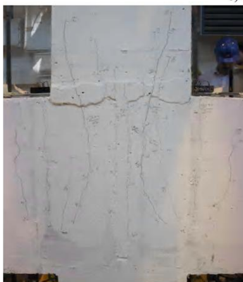
c) 105kN beam Load (prior to yielding)
