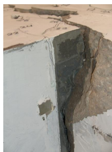
c) Left-bottom beam-column interface status at failure
