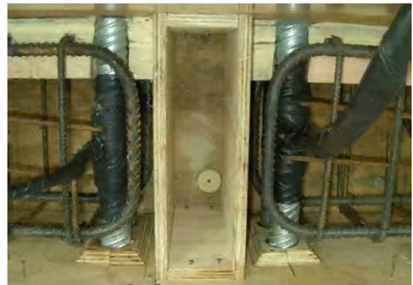
d ) Beam form work and beam-end reinforcement details of type T1 (specimens GR1 and SW1)
